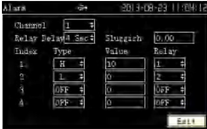
Alarm configuration Every channel can set four random alarm points.
