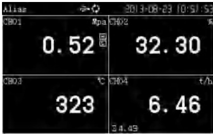
Digital display Measured values, channel number, engineering unit, alarm status and accumulative message,all of them will be displayed in digital form.
