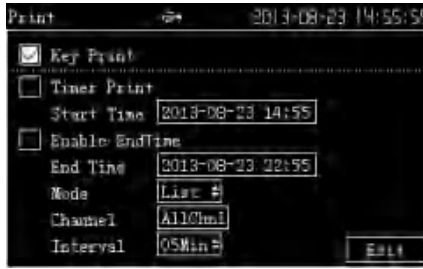
Print Configuration Setting button print and regular print, print real-time data for each channel.
